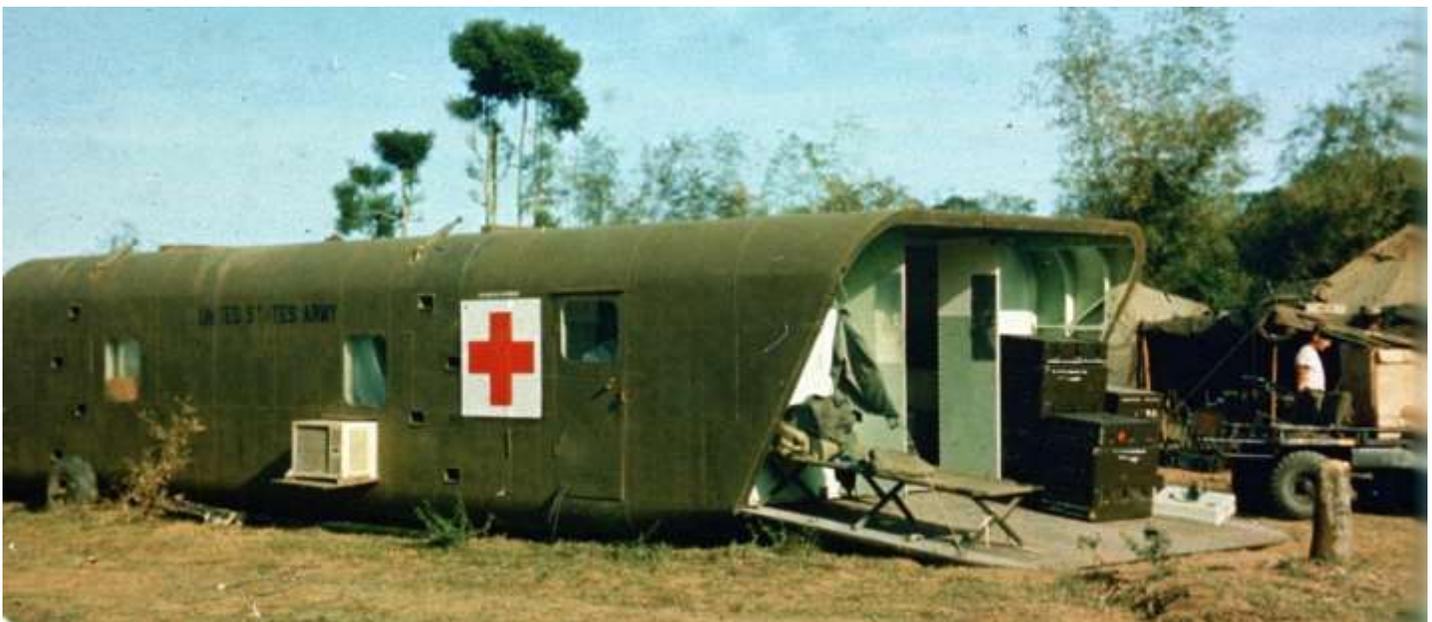
The CH-54 ‘Skycrane’ heavy lift helicopter allowed the AMEDD to experiment with air-lifted medical pods in the late 1950s through the mid-1960s. Everything from an aid station to an operating suite to a dental clinic could be moved wherever there was enough flat ground.
